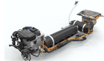
Hydrogen fuel cell & tank system
