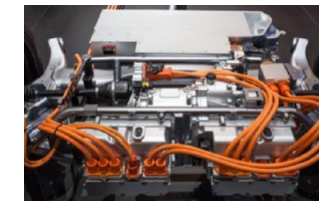
High voltage lines
